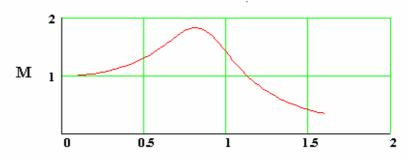
The result resembles the response of a second order system where the peak  $M_p=1.83$  and the resonant frequency is  $\omega_r=0.8\ rad/s$
