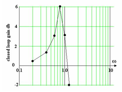
The peak magnification is at 0.8 rad/s and the closed loop gain is 6 db.
