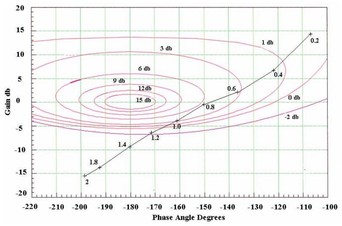
Now pick off the closed loop gain at various frequencies and plot the frequency response. It is typical of a second order system.
