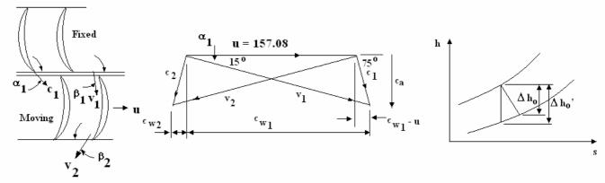
$$\begin{split} &u = \pi ND = \pi \ x \ 50 \ x \ 1 = 157.08 \ m/s \\ &\tan \alpha_1 = c_a/c_{w1} \\ &c_{w1} \tan 15 = (c_{w1} - u) \ \tan 75 \quad 0.269 \ c_{w1} = 3.732 (c_{w1} - 157.08) \\ &0.269 \ c_{w1} = 3.732 c_{w1} - 586.23 \\ &586.23 = 3.463 \ c_{w1} \\ &c_{w1} = 169.28 \ m/s \\ &c_{w2} = c_{w1} - u = 169.28 - 157.08 = 12.2 \ m/s \\ &c_a = c_{w2} \ \tan \beta_2 = 12.2 \ \tan 75 = 45.55 \ m/s \\ &\Delta \ c_w = 169.28 + 12.2 = 181.5 \ m/s \end{split}$$
