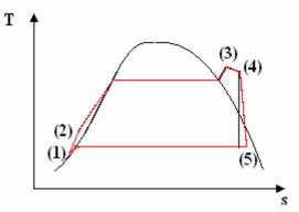
On the T –s diagram the water is under-cooled at (1)
