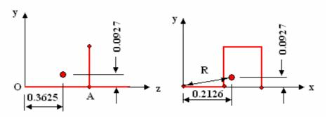
At the instant the torque is applied the angular velocity is zero so no centrifugal force is produced. If the body is free to rotate it will rest with the centre of gravity vertically below the z axis. Only the weight of the body acting at the centre of gravity need be considered. Taking moments about 'O' we have:
