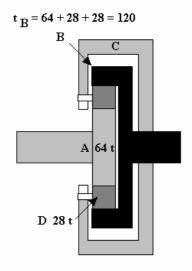
(a) With C stationary it not an epicyclic gear box but a simple gear train.
